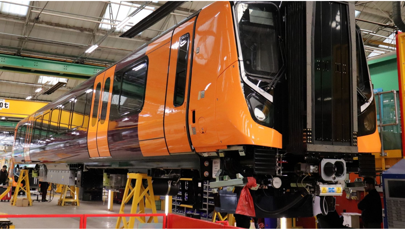
West Midlands Railway - Class 730 - Bombardier production line
